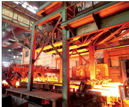
**Descaling of steel sheets and profiles.**
