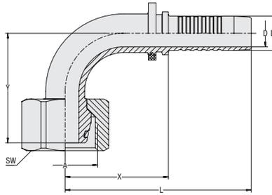
**Connection Type** Female Metric Nut Thread
