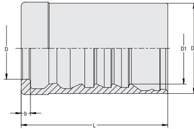
**Ferrule Type** with Pull-Out Protection (Interlock)
