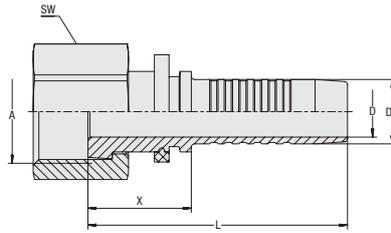
**Connection Type** Female UN/UNF Nut Thread
