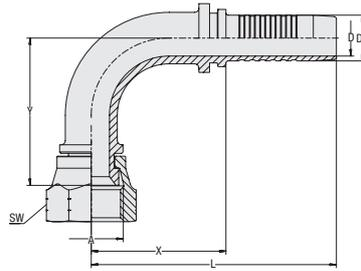
**Connection Type** Female UN/UNF Nut Thread
