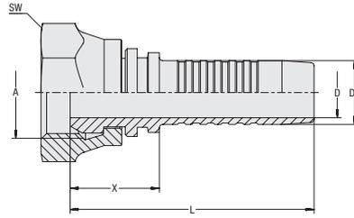
**Connection Type** Female BSPP Nut Thread
