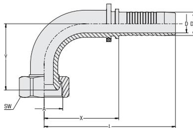
**Connection Type** Female Metric Nut Thread
