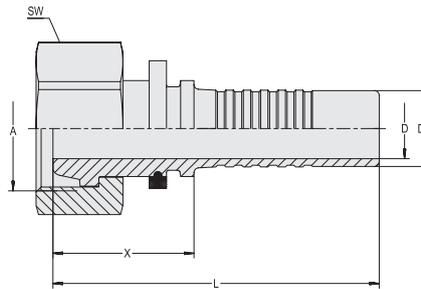
**Connection Type** Female Metric Nut Thread
