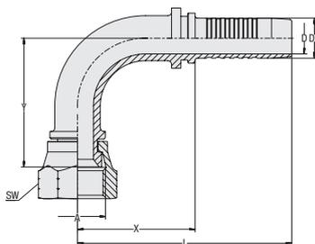
**Connection Type** Female BSPP Nut Thread
