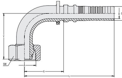
**Insert Type** with Pull-Out Protection (Interlock)
