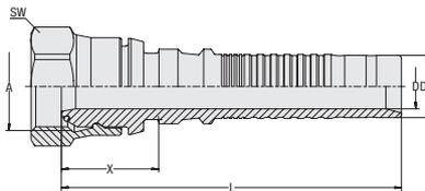
**Insert Type** with Pull-Out Protection (Interlock) for Hammer/Breaker Operation
