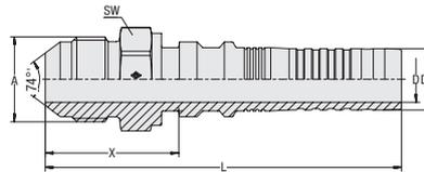
**Insert Type** with Pull-Out Protection (Interlock)
