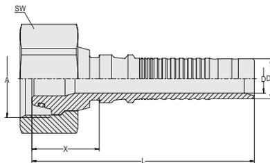
**Insert Type** with Pull-Out Protection (Interlock) for Hammer/Breaker Operation
