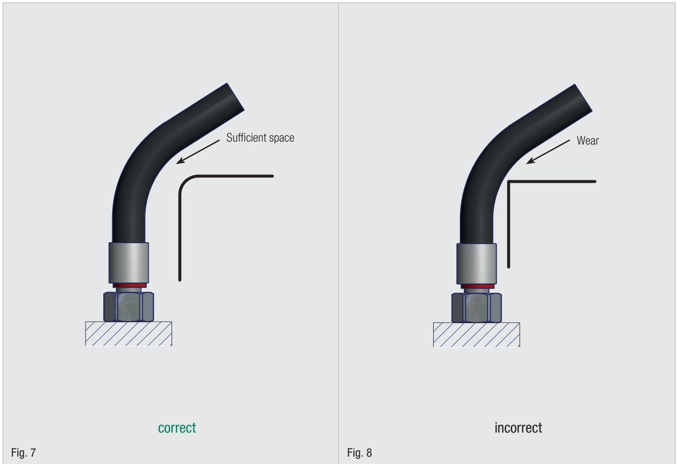
Avoid external mechanical effects on the hose, and prevent the hoses from rubbing against each other or other components, by installing and attaching them correctly (see Fig. 7).
