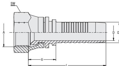
**Connection Type** Female BSPP Nut Thread
