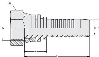
**Connection Type** Female UN/UNF Nut Thread
