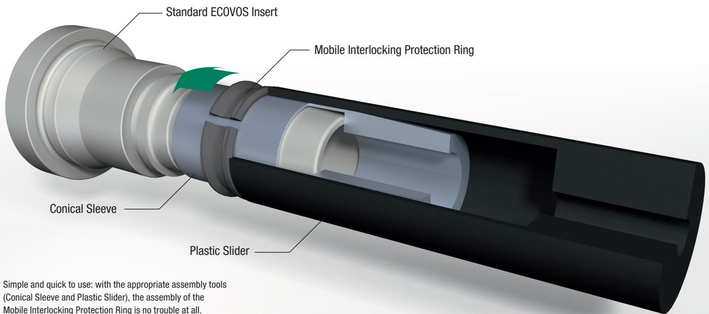
Simple and quick to use: with the appropriate assembly tools (Conical Sleeve and Plastic Slider), the assembly of the Mobile Interlocking Protection Ring is no trouble at all.
