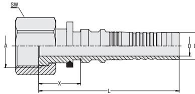
**Insert Type** with Pull-Out Protection (Interlock)
