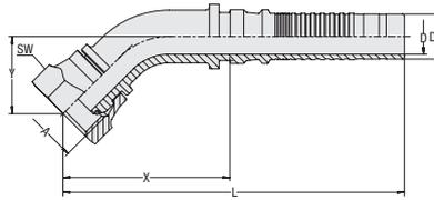
**Insert Type** with Pull-Out Protection (Interlock)
