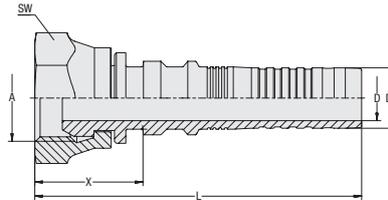
**Insert Type** with Pull-Out Protection (Interlock)
