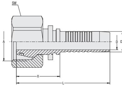
**Connection Type** Female Metric Nut Thread
