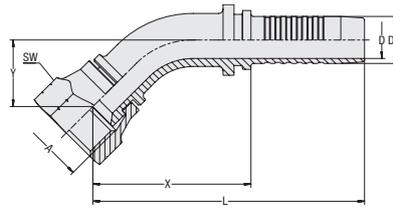
**Connection Type** Female Metric Nut Thread
