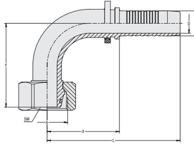
**Connection Type** Female Metric Nut Thread
