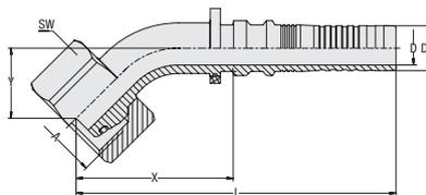
**Insert Type** with Pull-Out Protection (Interlock)
