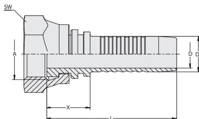
**Connection Type** Female BSPP Nut Thread
