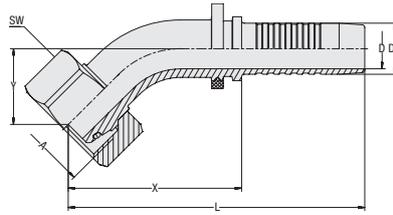
**Connection Type** Female Metric Nut Thread
