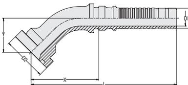
**Insert Type** with Pull-Out Protection (Interlock)
