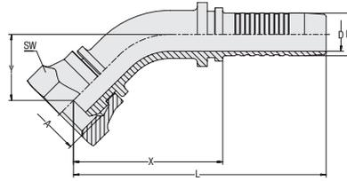
**Connection Type** Female BSPP Nut Thread
