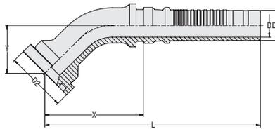
**Insert Type** with Pull-Out Protection (Interlock)
