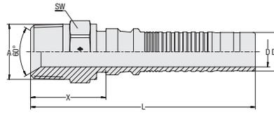
**Insert Type** with Pull-Out Protection (Interlock)
