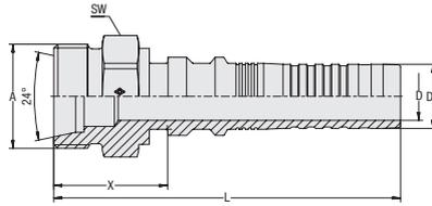
**Insert Type** with Pull-Out Protection (Interlock)
