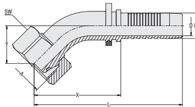
**Connection Type** Female Metric Nut Thread
