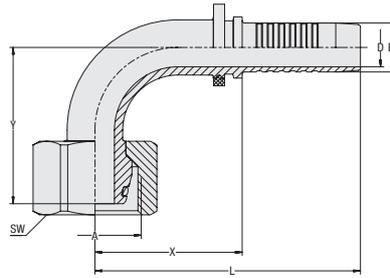
**Connection Type** Female Metric Nut Thread
