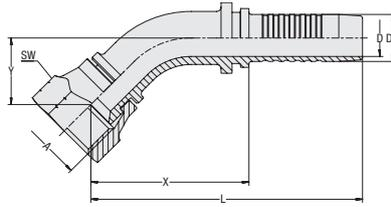
**Connection Type** Female UN/UNF Nut Thread
