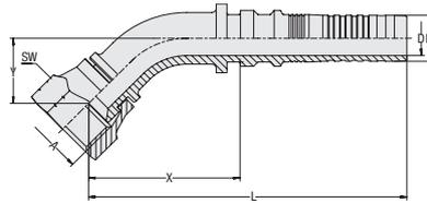
**Insert Type** with Pull-Out Protection (Interlock)
