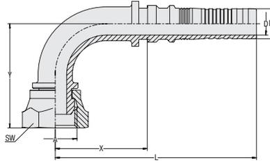
**Insert Type** with Pull-Out Protection (Interlock)
