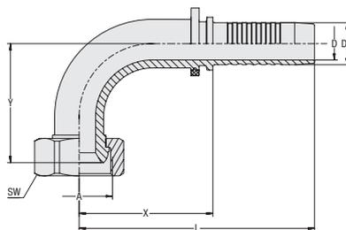
**Connection Type** Female Metric Nut Thread
