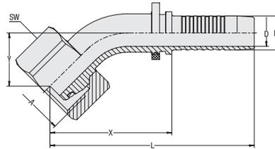
**Connection Type** Female Metric Nut Thread
