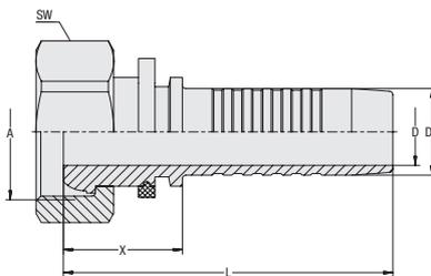
**Connection Type** Female Metric Nut Thread
