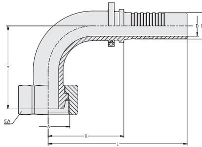
**Connection Type** Female Metric Nut Thread
