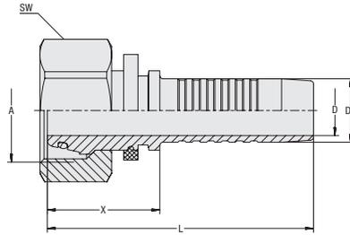
**Connection Type** Female Metric Nut Thread
