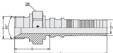
**Insert Type** with Pull-Out Protection (Interlock)
