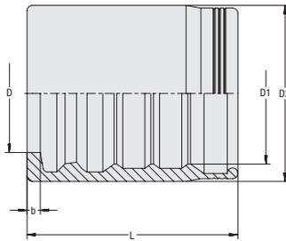
**Ferrule Type** with Pull-Out Protection (Interlock)
