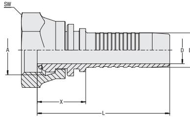
**Connection Type** Female BSPP Nut Thread
