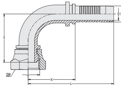
**Connection Type** Female BSPP Nut Thread
