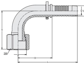
**Connection Type** Female UN/UNF Nut Thread
