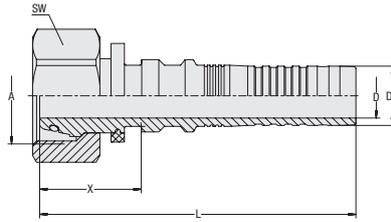
**Insert Type** with Pull-Out Protection (Interlock)
