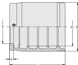
**Suitable for Standard** 1SC, 2SC, 1SN-K, 2SN-K
