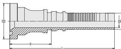
**Insert Type** with Pull-Out Protection (Interlock)
