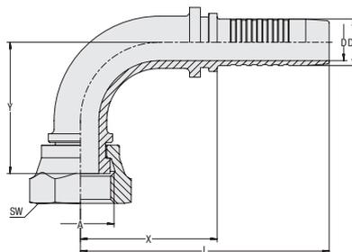
**Connection Type** Female BSPP Nut Thread
