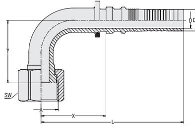
**Insert Type** with Pull-Out Protection (Interlock)
