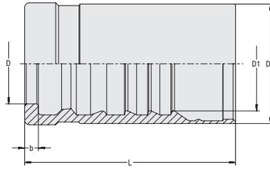
**Ferrule Type** with Pull-Out Protection (Interlock)
