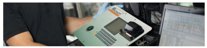
With measuring, testing, display and analysis devices and equipment from the STAUFF Diagtronics product range, system operators, maintenance personnel and repair technicians can determine and monitor the essential parameters in mobile and industrial hydraulics: operating pressure, maximum pressure, differential pressure, system temperature, volume flow, contamination and much more.
